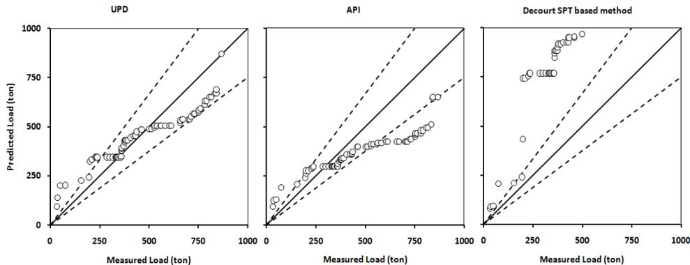
Fig. 6 predicted capacity versus measured capacity for different methods
