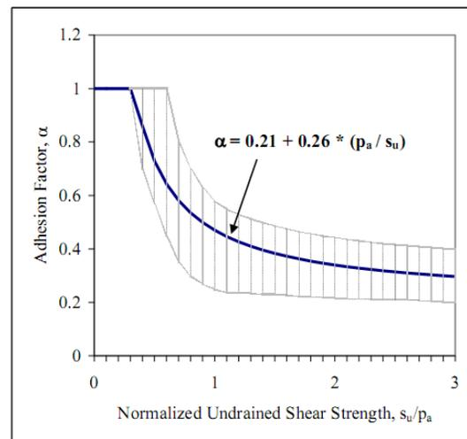
Fig. 4 Variation of  $\alpha$  with  $c_u/p_a$  based on tested results by Kulhawy and Jackson (1989) [23]
