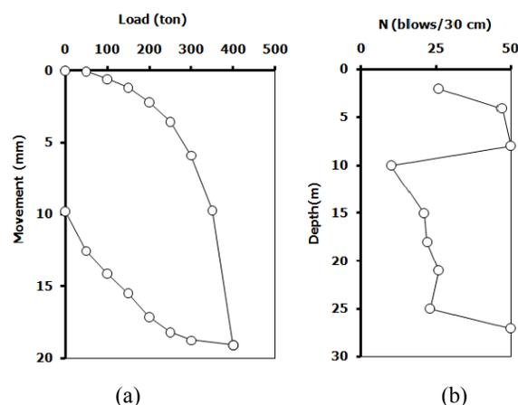
Fig. 2 A typical case records pile load test (a).SPT test result in Khalij-e Fars Ship Yard project (A1-122a pile) (b).
