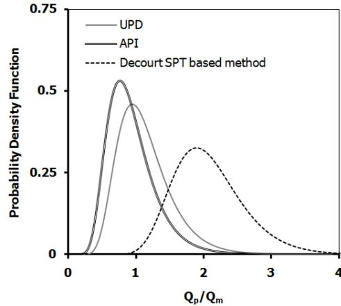
**Fig. 8** Log-Normal Probability curve for different methods
