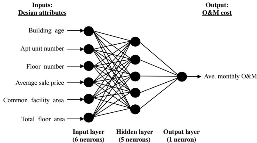
Fig. 1 The neural network architecture for predicting O&M costs of condominium properties.
