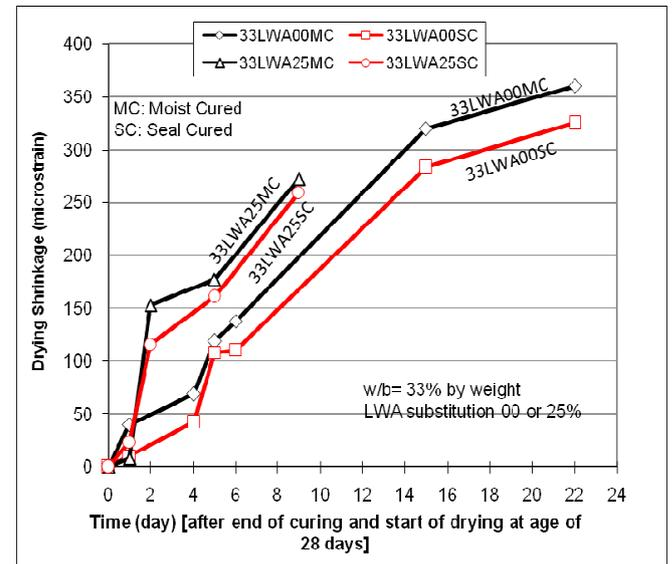
Fig. 9. Drying shrinkage vs. drying time of SCC mixtures after 28 days of moist and sealed curing
