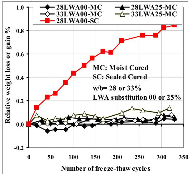
Fig. 10. Relative values of weight loss or gain of specimens subjected to freezing and thawing
