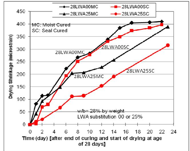
Fig. 8. Drying shrinkage vs. drying time of SCC mixtures after 28 days of moist and sealed curing
