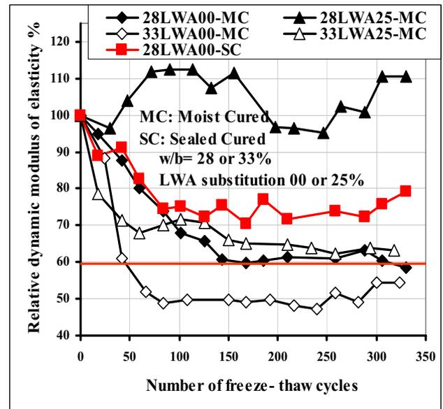
Fig. 11. Relative dynamic modulus of elasticity vs. number of freeze/thaw cycles
