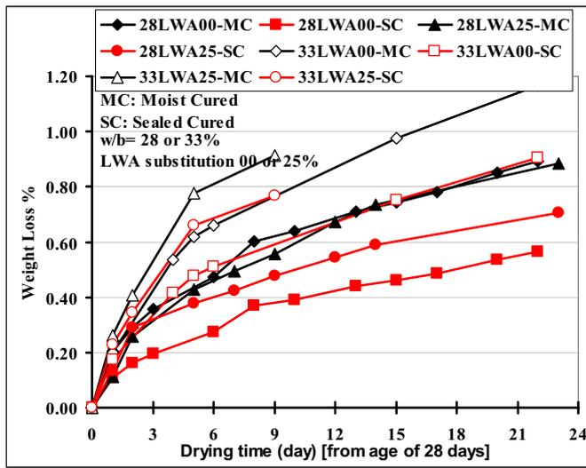
Fig. 6. Weight loss relative to the first weight measurement vs. time after drying started
