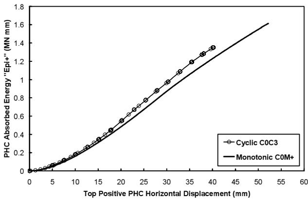
Fig. 9. PHC absorbed energy calculated for cyclic and monotonic loading
