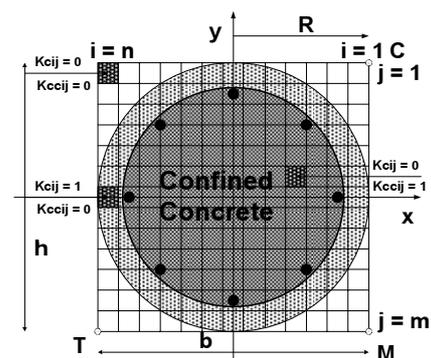
Fig. 1. Discretization of a RC member's section
