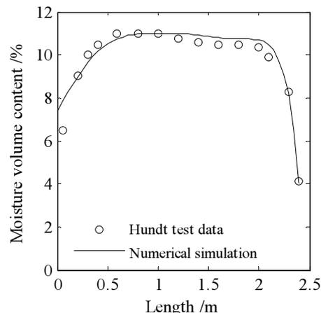
Fig.8. Comparison of numerically and experimentally moisture distribution (550d)
