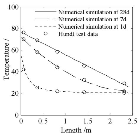
**Fig.9.** Comparison of numerically and experimentally temperature distribution
