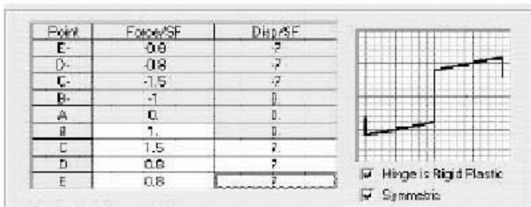
Figure 2-B: Nonlinear plastic Hinge Shear
