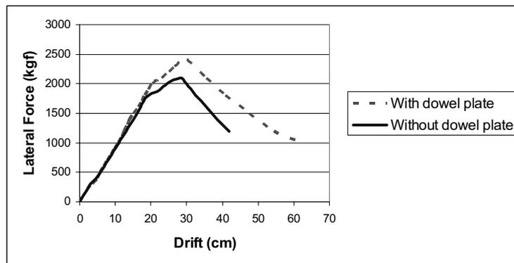
Fig.9 Effect of dowel plates on pushover diagram
