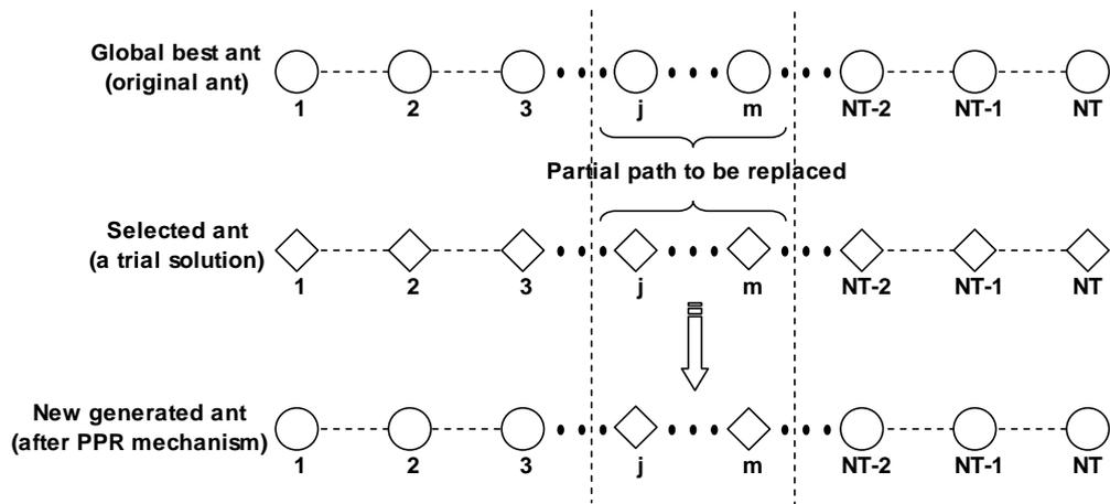
Fig. 1 Schematic of Partial Path Replacement (PPR) Mechanism
