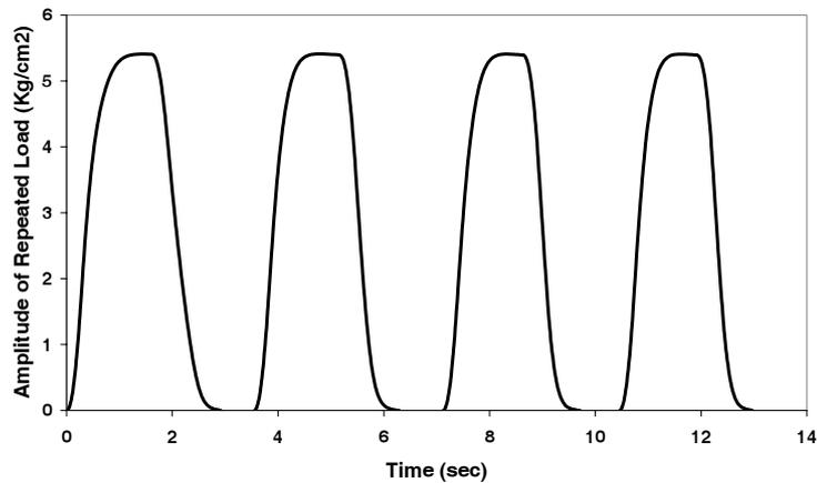
Fig. 2. Time history of repeated load on the soil surface.
