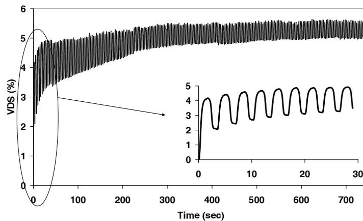
Fig. 3. Typical trend of VDS during repeated loads.
