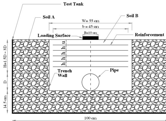
Fig. 1. The schematic layout of the trench.
