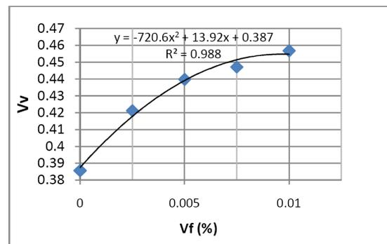
Fig. 3. Voids Volume Relation versus PP Fiber Fraction
