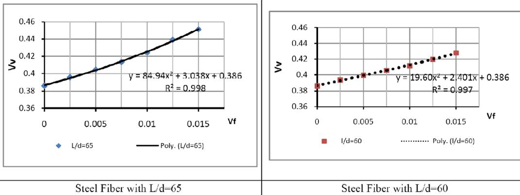
Fig. 2. Voids Volume Relation versus Steel Fiber Fraction
