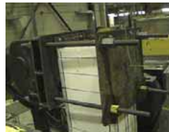
Fig.3 Locations of LVDT's and the Test Setup for Beams
