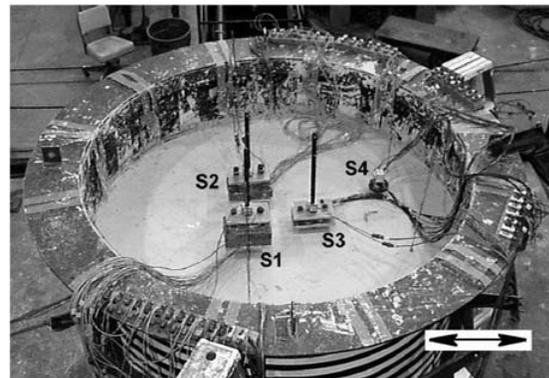
Fig. 1 Configuration of Shaking Table Test [10].
