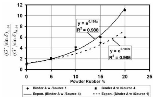
**Fig. 2** Determination of Rubber Coefficient for  $G^*/\sin \delta$ .
