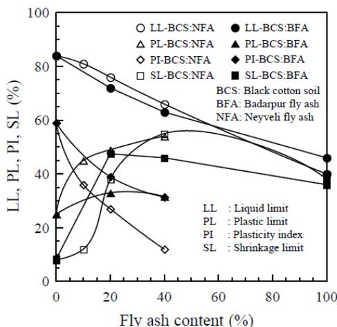
Fig. 4 Effect of fly ash on index properties of BC soil
