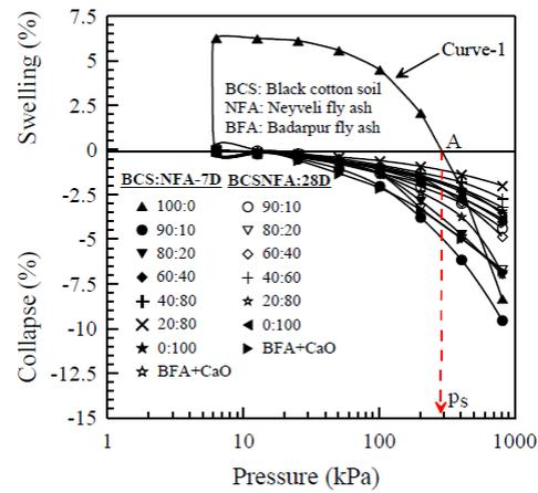
Fig. 7(b) Effect of Neyveli fly ash on swelling & collapse characteristics of BC soil
