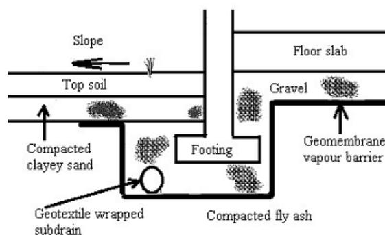
Fig.2 (b) Building foundation using fly ash
