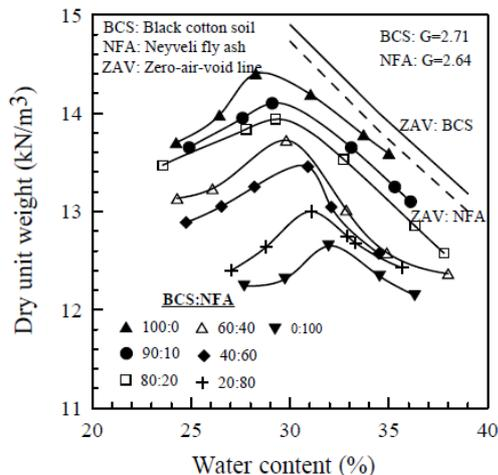
Fig. 5(b) Effect of Neyveli fly ash on compaction characteristics of BC soil
