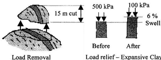
Fig. 1(a) Volume change of BC Soil due to removal of load
