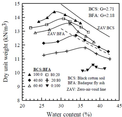
Fig. 5(a) Effect of Badarpur fly ash on compaction characteristics of BC soil
