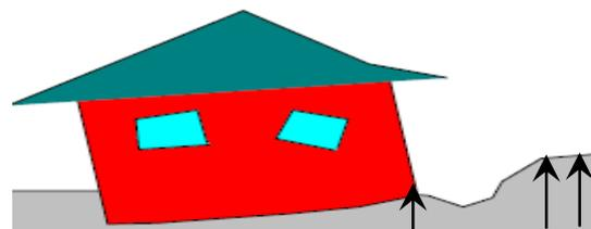
Fig. 1(b) Localized heave due to drainage problems
