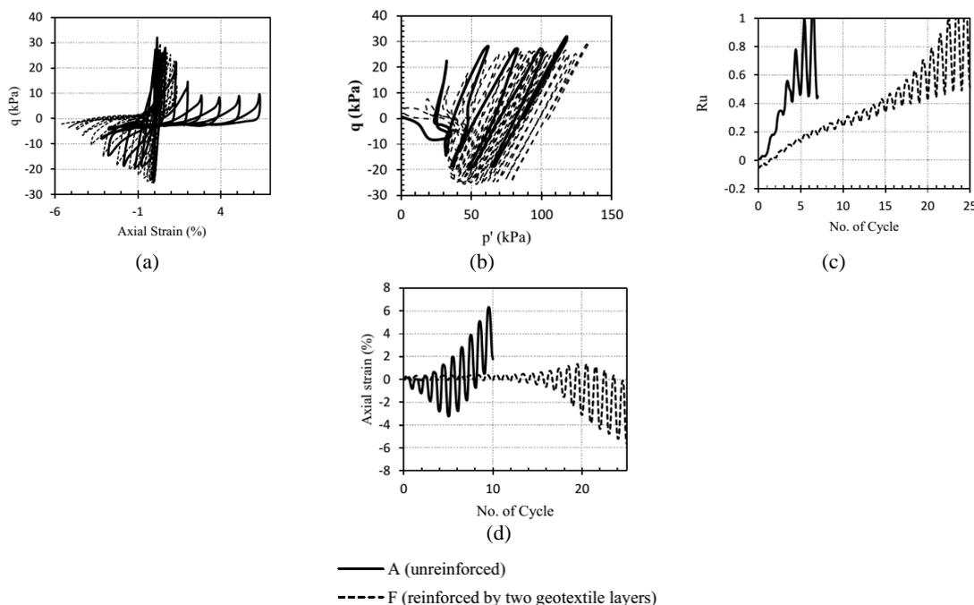
**Fig. 3** Comparison of cyclic test results of unreinforced (A) and reinforced silty sand (10% silt) samples (F arrangement)  $CSR=0.275$
