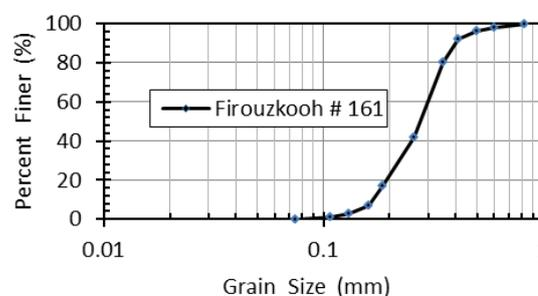
**Fig. 1** Grain size distribution curve of Firouzkuh #16 sand
