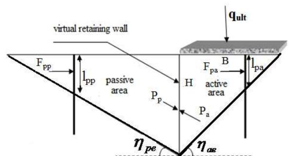
Fig. 5 Failure mechanism in reinforced soil with piles
