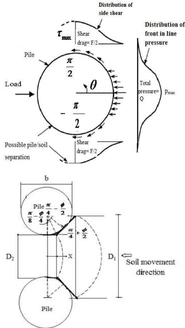
Fig. 4 Lateral resistance of soil around piles
