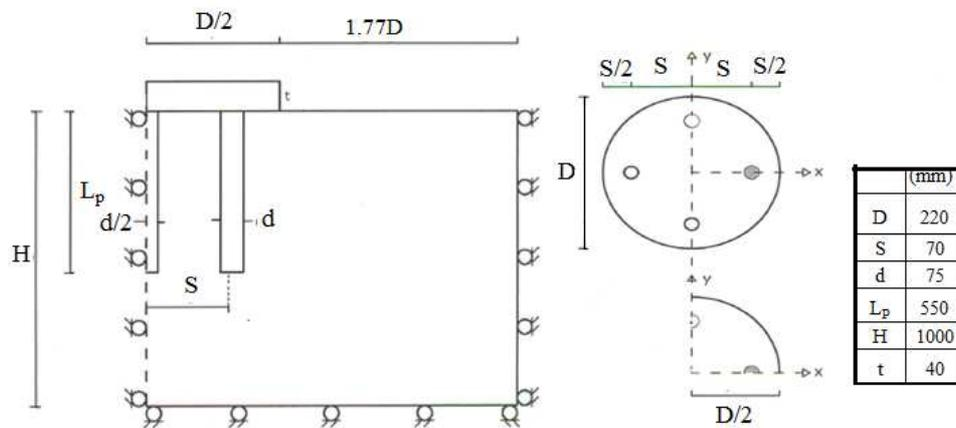
**Fig. 11** Physical model geometry of Baziar et. al [12]
