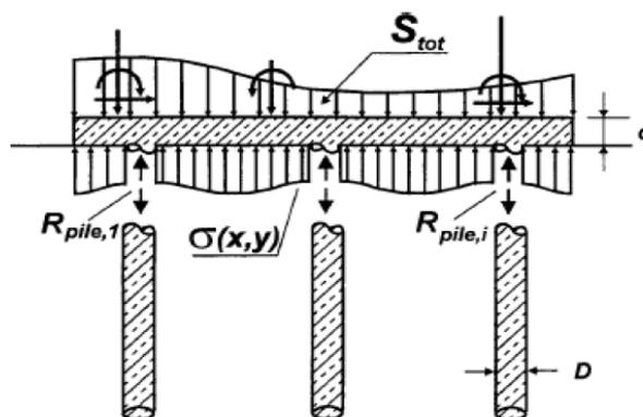
Fig. 1 Interaction between pile, soil and foundation
