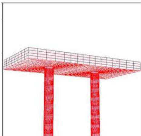
**Fig. 7** Using interface elements around pile and footing
