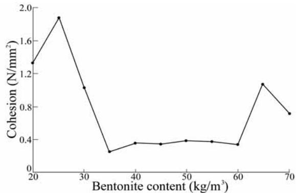
Fig. 7. Effect of bentonite content on cohesion.
