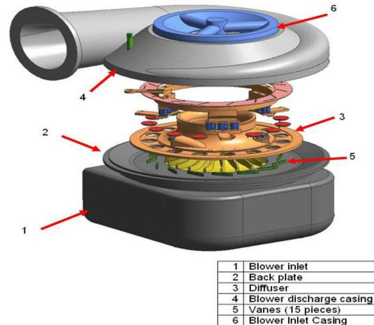
**Fig. 1.** Complete extrusion of the VGT compressor
