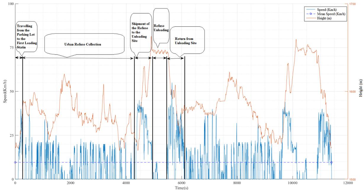
**Figure 4:** Speed and height versus time graph of refuse collection truck within half a working day
