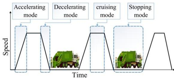
**Figure 1:** Pattern of the refuse collection driving cycle
