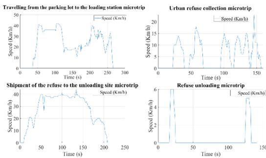
**Figure 5:** An example of the representative micro trips for the clusters.
