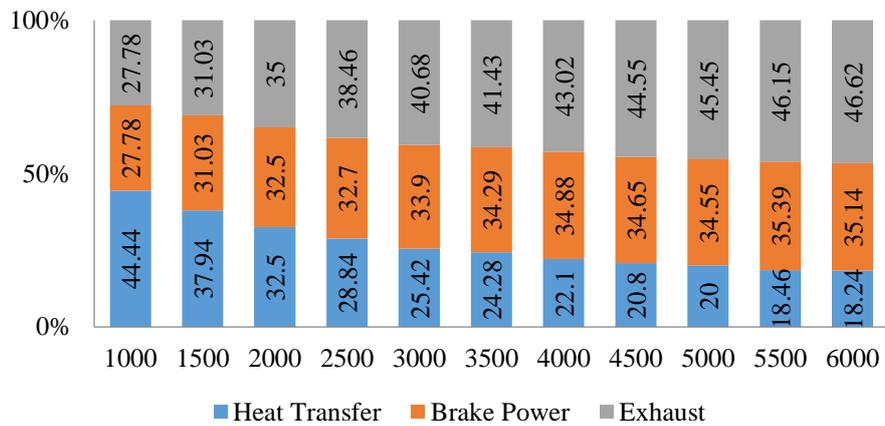
Figure 10: Energy Distribution of in Different Engine Speeds
