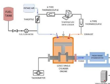
**Figure 1:** Schematic Diagram of Engine Test Setup
