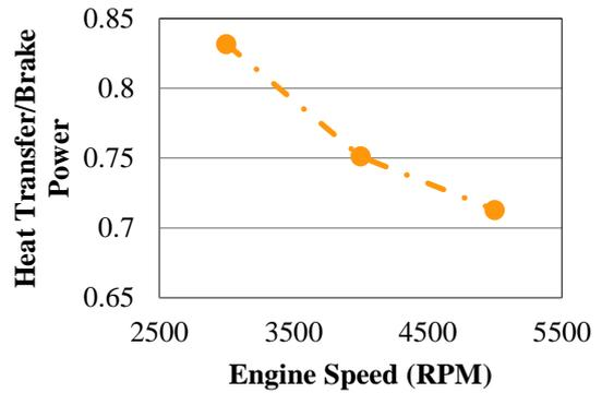
Figure 9: Experimental Heat Transfer to Brake Power Ratio
