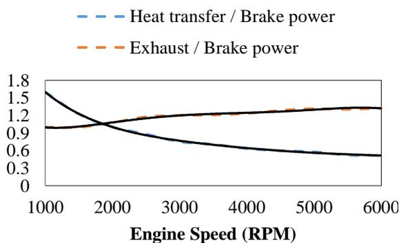
Figure 12: Energy Distribution of in Different Engine Speeds
