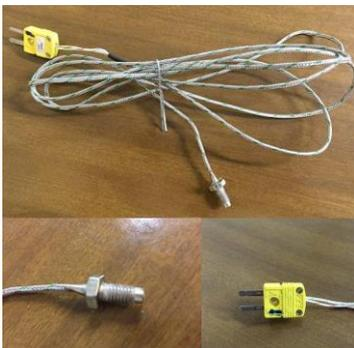
**Figure 2:** Sample Thermocouple and Its Wire and Socket
