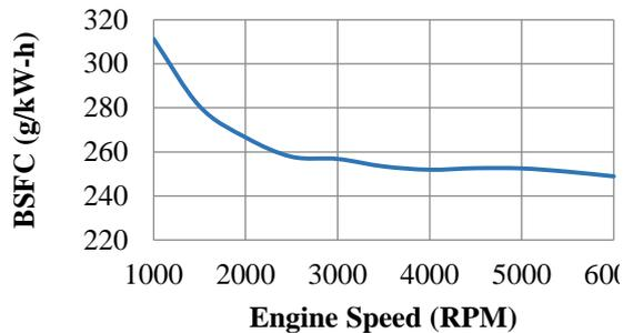
**Figure 13:** Brake Specific Fuel Consumption in Different Engine Speeds
