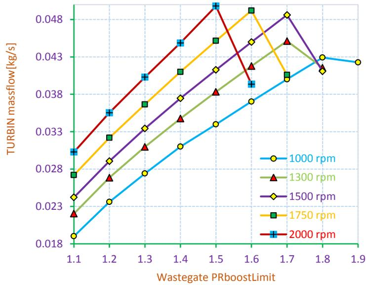
Fig12. Turbine mass flow comparison at different speeds.
