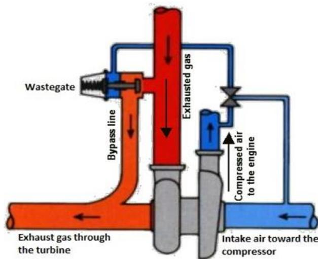
Fig1. Schematic diagram of exhaust WASTE GATE
