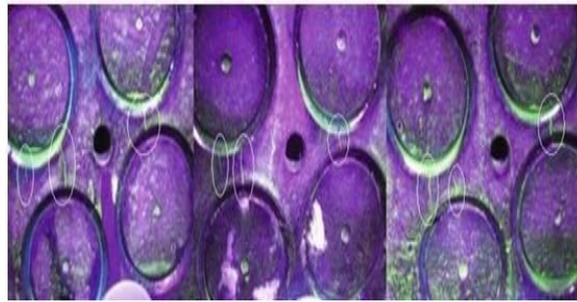
Fig12. The cracked diesel engine cylinder head [11].
