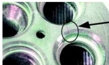
Fig11. The cracked diesel engine cylinder head [19].
