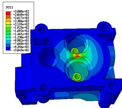
Fig4. The temperature distribution in the cylinder head
