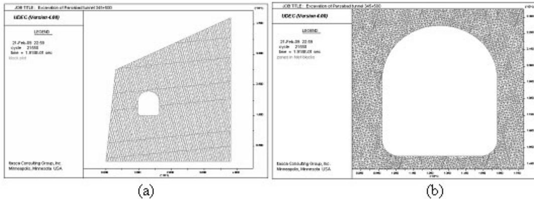
Fig. 4. (a) Geometry of the section chosen for dynamic analysis (b) mesh generation around the tunnel.
