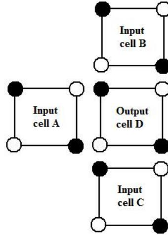
Figure 5. the input cells and output cells of a majority voting gate.
