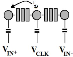
Figure 2. When the clock signal is on, electron tunnels to the dot with positive potential
