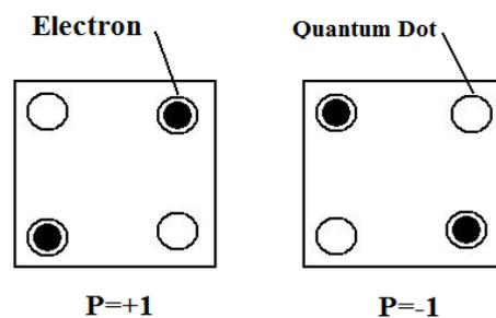
Figure 1. standard QCA cells showing the polarizations of two ground states.
