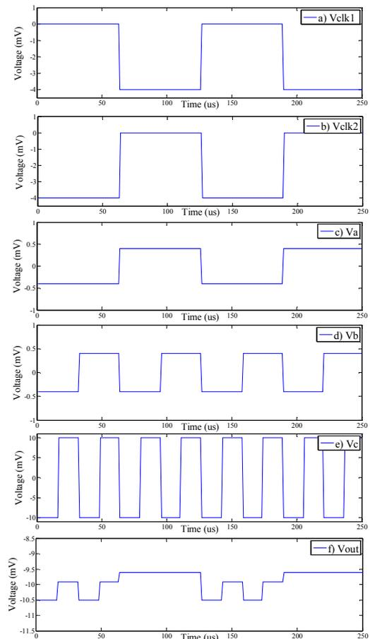
Figure 6. Simulation results of a clocked QCA majority gate. (a) clock voltage of left half of circuit. (b) clock voltage of right half of circuit. (c) output voltage of input cell A. (d) output voltage of input cell B. (e) output voltage of input cell C. (f) output voltage of output cell D.
