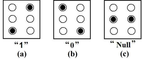
Figure 3. A clocked QCA cell that is a six-dot cell.(b) varying the potential of the middle dots or pulling the electrons onto the middle dots leads to a “null” state of the cell, (a), (c) and by varying the potential of the middle dots or by pushing the electrons off of the middle dots state of the cell become “1” or “0”.
