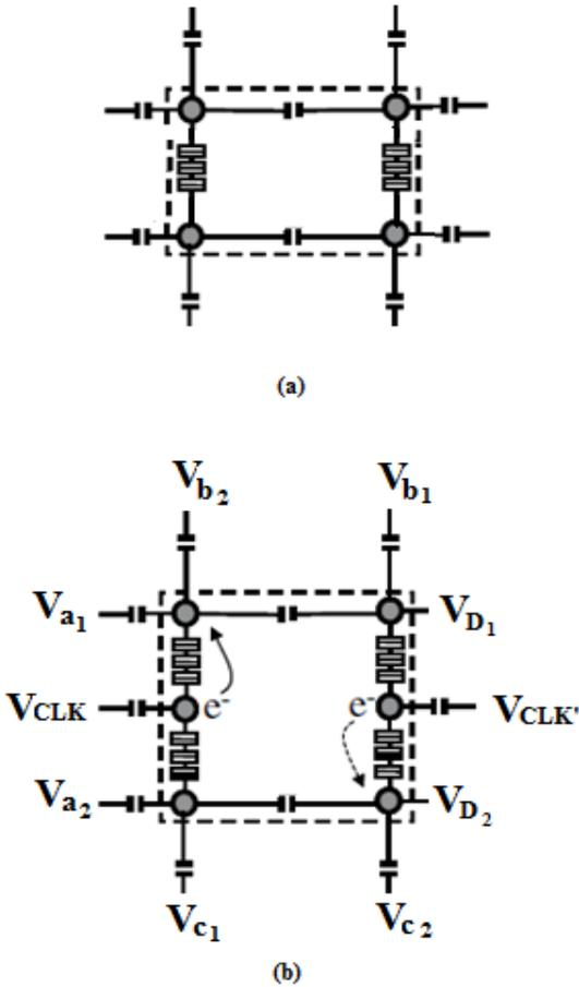
Figure 4.(a) A Realization of a basic QCA cell composed of quantum dots, tunnel junctions and capacitances. (b) Schematic diagram of a clocked three-input majority gate circuit.
