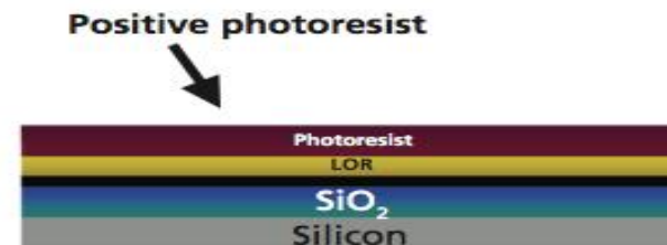
c) Deposit lift-off resist and photoresist
