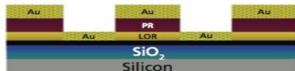
g) Evaporate gold onto substrate
