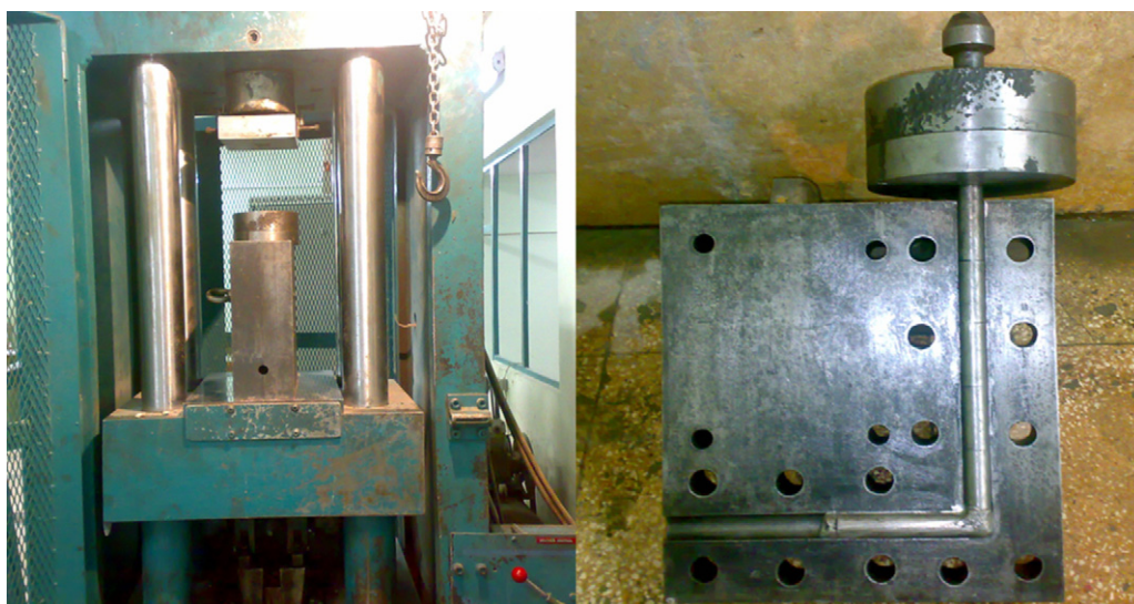
Fig. 4. The ECAP set-up for experimental work: hydraulic press and ECAP die set-up.
