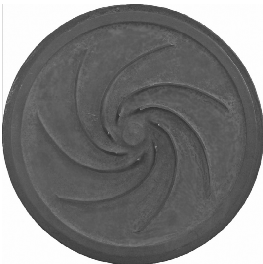
Fig. 6. Impeller of Berkeh 32-160 pump.
