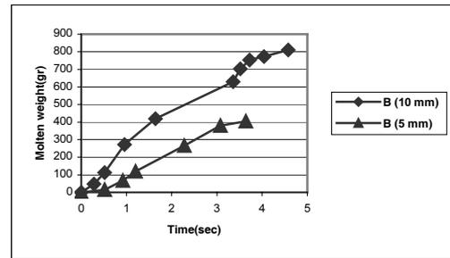
Fig. 12. Effect of the pattern geometry on mold filling in bottom gating system
