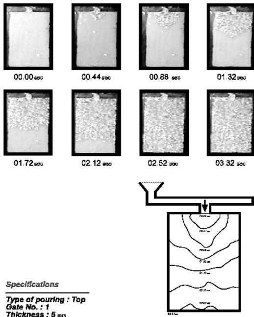
**Fig. 3.** Mold filling sequences in the top pouring of a 5 mm thick plate in the LFC process
