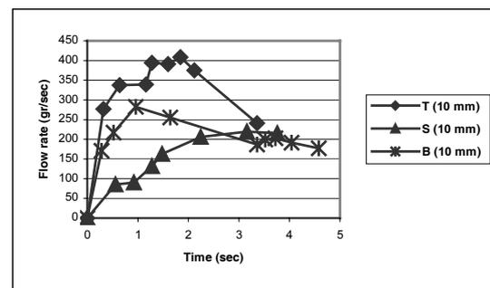
**Fig. 18.** Effect of the gating system on mold filling in 10 mm thickness
