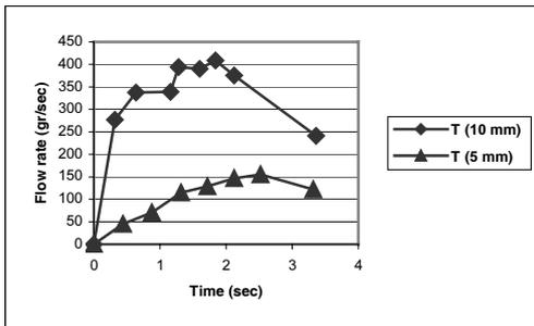
Fig. 11. Effect of the pattern geometry on mold filling in top gating system
