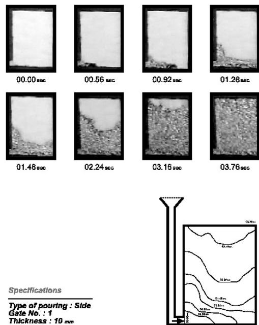
**Fig. 6.** Mold filling sequences in the side pouring of a 10 mm thick plate in the LFC process
