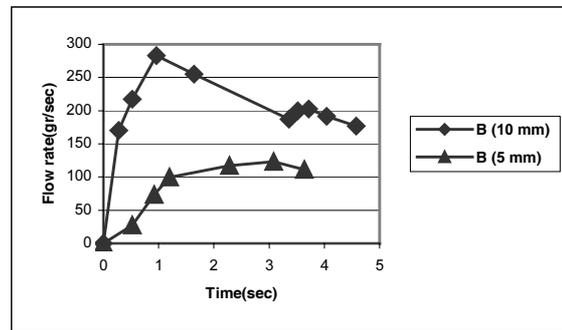
Fig. 14. Effect of the pattern geometry on mold filling in bottom gating system
