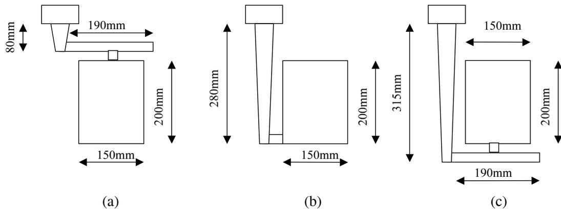
**Fig. 1.** Schematic illustration of the gating systems: (a) top gating. (b) side gating (c) bottom gating
