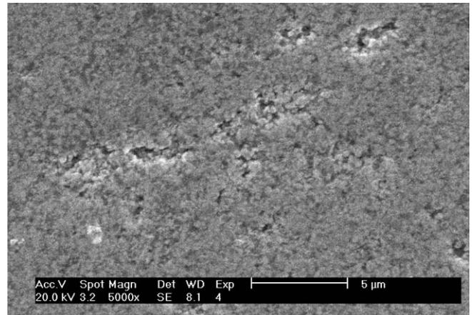
Fig. 8. SEM micrograph of the samples sintered at 1000 °C for 1.5 h.
