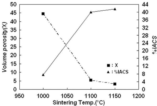
Fig. 10. The effect of sintering temperature on conductivity (reported as percentage of International Annealed Copper Standard) and volume porosity of the sintered samples.
