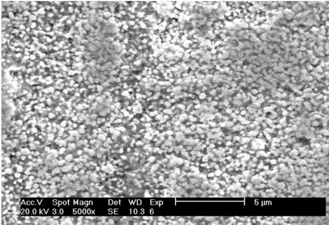
Fig. 9b. SEM image of the sintered samples at 1150 °C.
