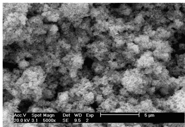
Fig. 4. SEM micrograph of the calcined powders at  $500\text{ }^{\circ}\text{C}$ .
