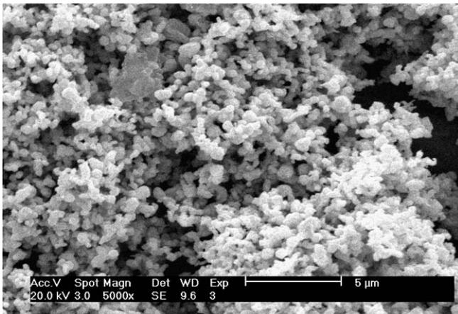
Fig. 6. SEM micrograph of the reduced powders.
