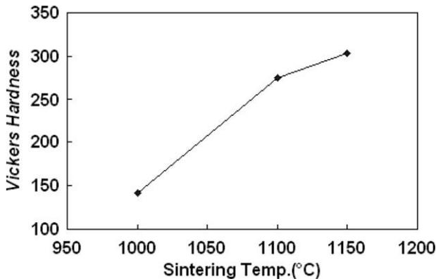
Fig. 11. Vickers hardness versus sintering temperature for the samples sintered at different temperatures.
