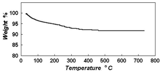
Fig. 2. TG curve of the initial precipitates up to  $750\text{ }^{\circ}\text{C}$  in air.
