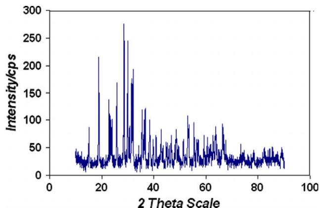
Fig. 3. XRD pattern of the calcined powders at  $500\text{ }^{\circ}\text{C}$ . The pattern shows only  $\text{CuWO}_{4-x}$  peaks.
