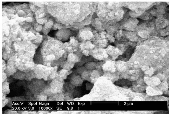
Fig. 1. SEM micrograph of the initial dried precipitates.
