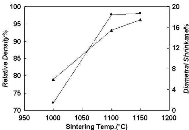
Fig. 7. Relative densities and diametral shrinkages of the samples versus sintering temperature. The theoretical density is  $14.33 \text{ g cm}^{-3}$ .
