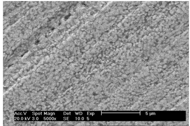
Fig. 9a. SEM image of the sintered samples at 1100 °C.
