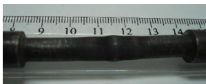
Fig. 9. Flow localization in the G4 specimen deformed at 1100°C and \omega = 10 rad.sec-1 after applying the reheating cycle
