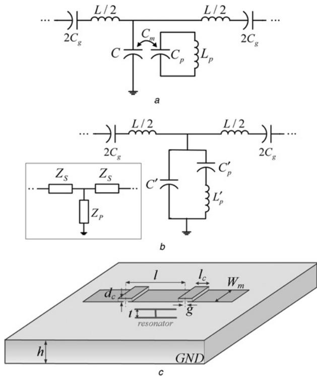
**Fig. 4** Lumped element equivalent circuit for the basic DN unit cell
