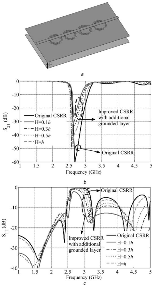
**Fig. 2** Layout of four improved CSRR structure with additional grounded layer to form a new continuous ground
