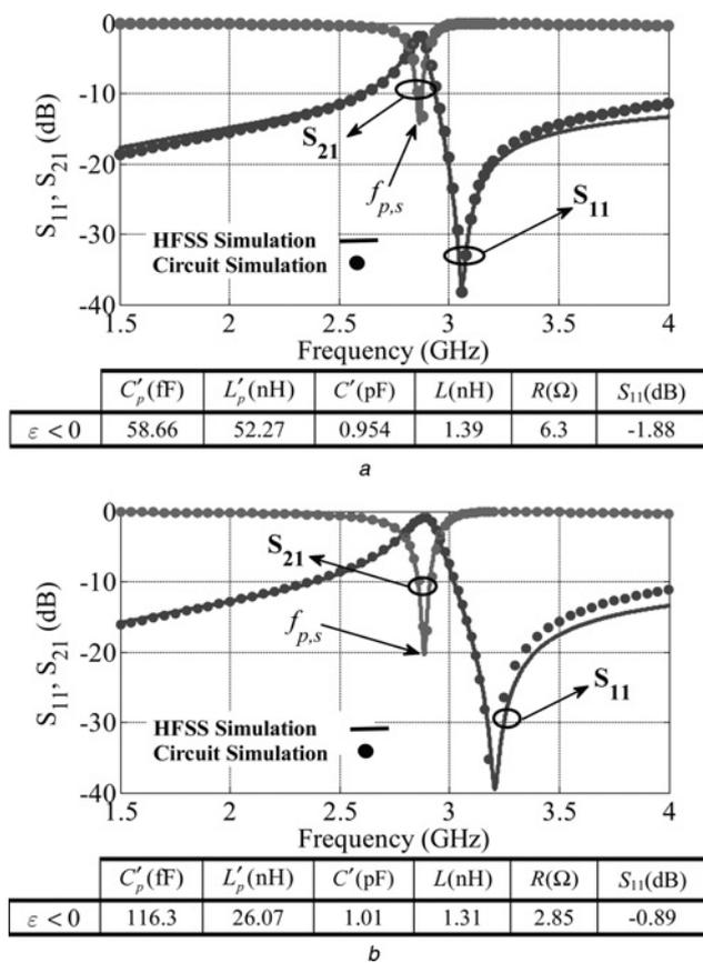
**Fig. 8** Frequency response (reflection,  $S_{11}$ , and transmission,  $S_{21}$ , coefficients) depicted in a decibel scale and extracted element parameters for two BC-SR resonators with dimensions
