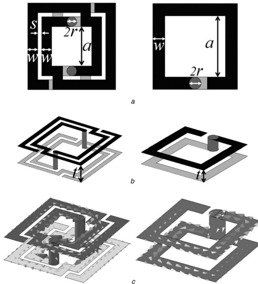
**Fig. 1** Topologies for metamaterial resonators with two metal levels (at both sides of a dielectric layer) connected by vias
