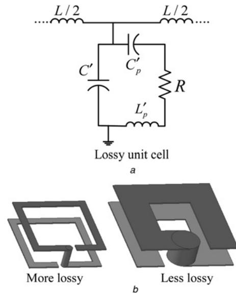
**Fig. 7** Lumped element equivalent circuit for the lossy unit cell (losses can be taken into account by including a series resistance in the model)
