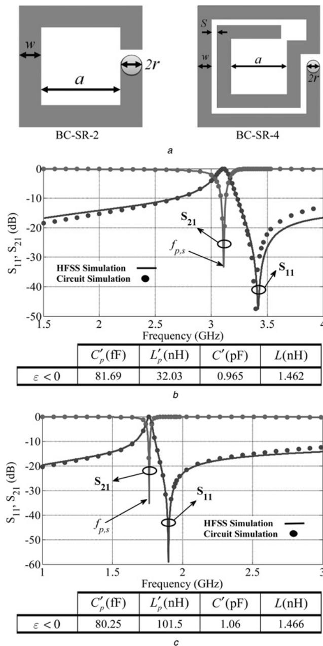
**Fig. 9** Topologies of the different resonators considered: BC-SR2 and BC-SR4
