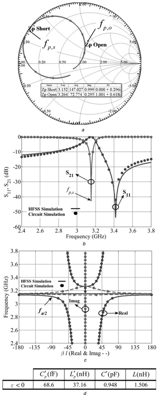
Fig. 5 Reflection coefficient on the Smith chart
