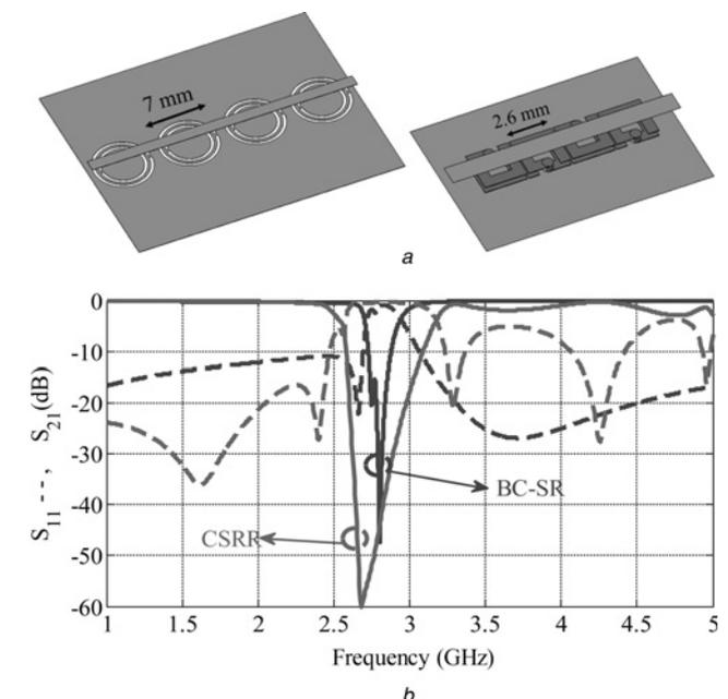
**Fig. 3** Layout of four BC-SRs and four CSRRs
