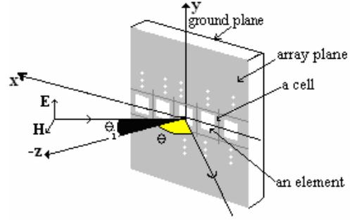
Fig. 1  $TE_z$  wave incidence
