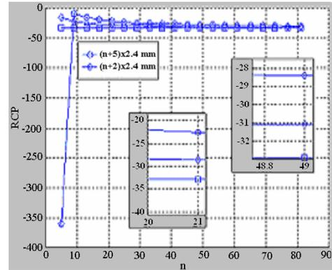
Fig. 2 RCP convergence in normal incidence versus  $n$
