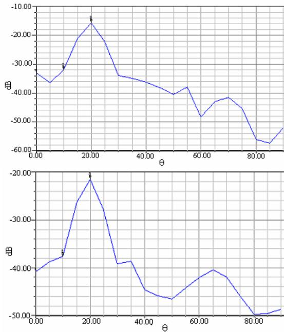
**Fig. 10** the E plane patterns of  $15 \times 15$  MRAs, designed one, the one composed of identical rectangular  $1.58 \times 1.3 \text{mm}^2$  elements and the one composed of identical square elements with side length of 1.3mm, respectively
