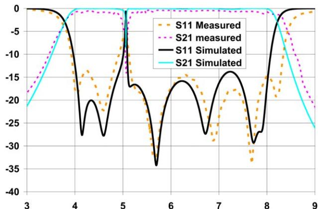
**Figure 8** Measured performance of the filter with one transmission zero in the passband. [Color figure can be viewed in the online issue, which is available at [wileyonlinelibrary.com](http://wileyonlinelibrary.com)]
