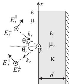
Figure 1. A typical homogeneous chiral slab exposed to an incident plane wave with an arbitrary linear combination of TM ( $E_i^{\parallel}$ ) and TE ( $E_i^{\perp}$ ) polarizations.
