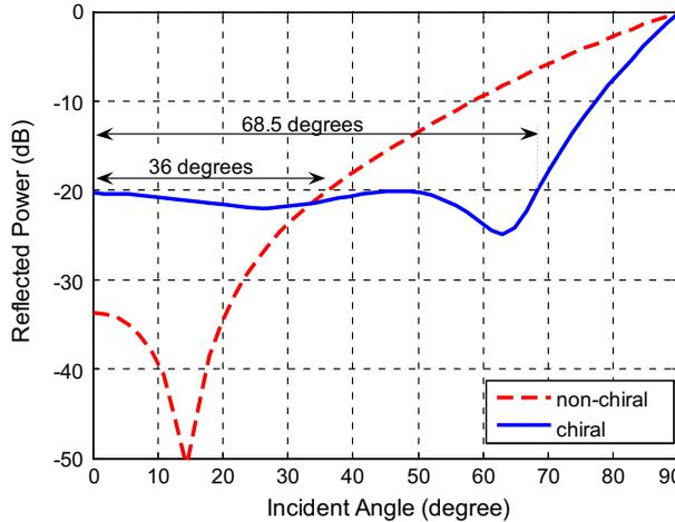
Figure 3. Coreflected power for PEC-backed inhomogeneous chiral and nonchiral slab.
