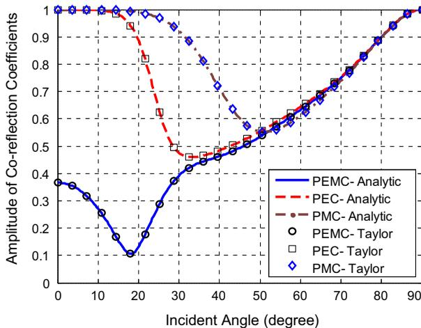
Figure 2. Coreflection coefficients for PEC-, PMC-, and PEMC-backed (with  $M = 0.01$ ) chiral slab.
