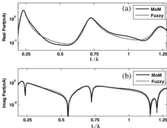
**Figure 7.** Comparing the modeled results of induced current by MoM and Fuzzy. (a) Real part, (b) imaginary part.
