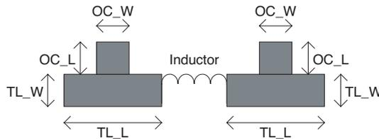
**Figure 1.** Equivalent circuit for branches of conventional Wilkinson.
