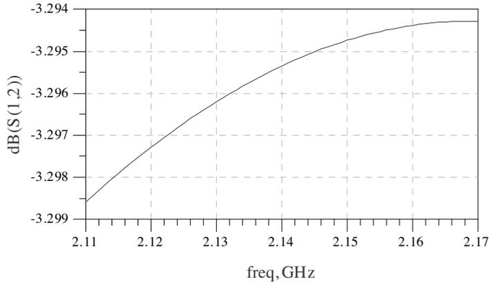
**Figure 7.** Coupling factor at desired frequency bandwidth.
