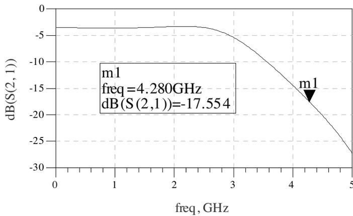
Figure 6. Coupling factor at wide frequency band.
